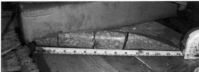
Figure 9. Curved outer surface retrieved from hidden pile by coring.
