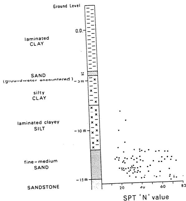
Figure 2 Simplified borehole log
