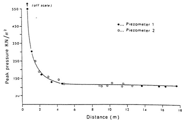
Figure 7 Peak pore pressures measured in Lower Sand during pile driving
