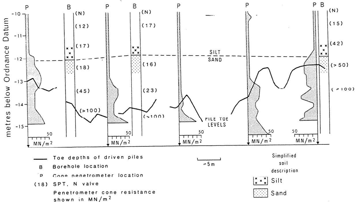
Figure 6 Toe depths for one line of piles together with relevant ground investigation data
