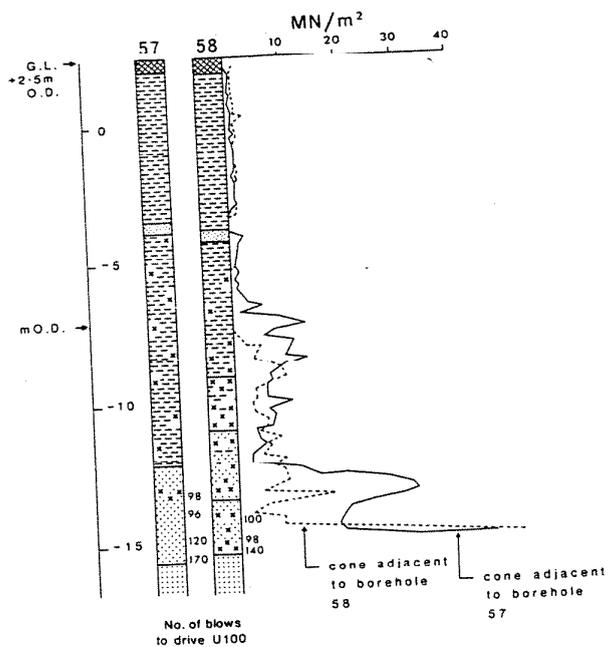
Figure 8 Ground conditions for groups of shallow (B57) and deep (B58) piles
