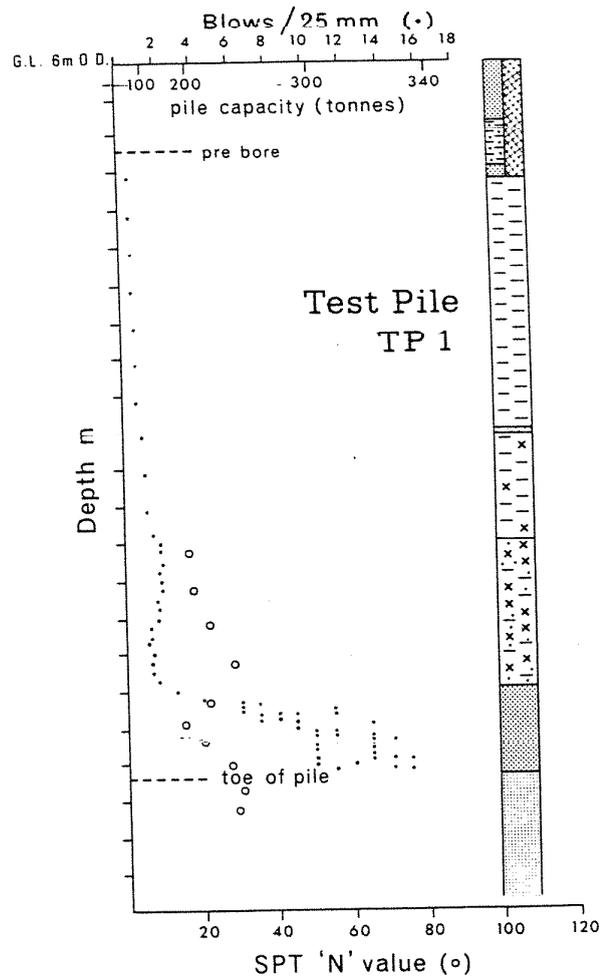
Figure 3 Details of test pile TP1
