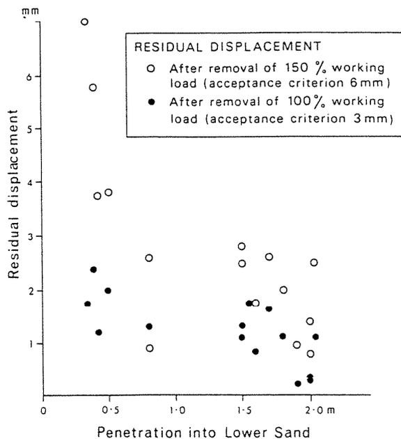
Figure 4 Residual settlements for piles penetrating different distances into the Lower Sand
