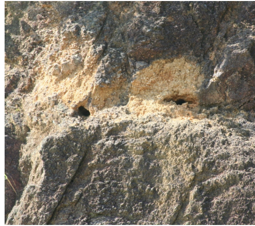
Figure 4. Natural pipes at interface between Grade V and Grade IV granite, Hong Kong
