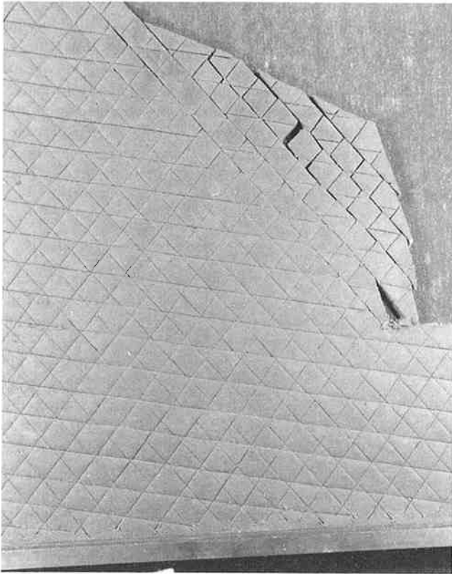
Fig. 2 Base-friction model of slope failing by sliding on daylighting discontinuities
