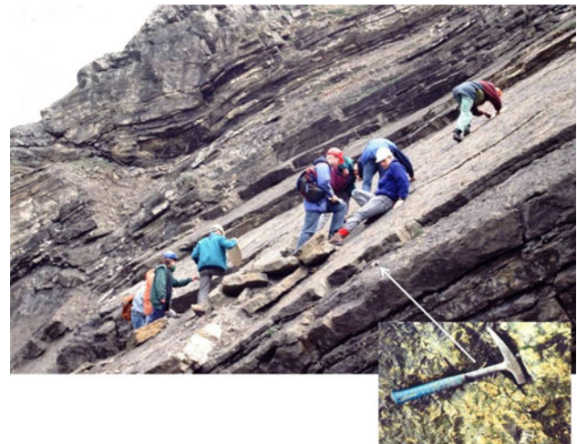
Fig. 18 Roughness survey under way using plates of different diameter on a bedding plane discontinuity in shaley limestone (Skipton, Yorkshire). At the small scale (hammer) the joint is rough but at larger scale the joint is effectively flat
