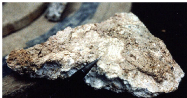
Fig. 20 Hard, slickensided kaolinite infill from downwarp on failed sheeting joint (Hencher 1983). Pencil for scale
