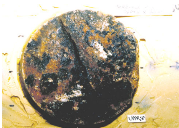
Fig. 19 Sample V13, 8.7 m (North Point Study, Hong Kong) following 5 stage, repeated direct shear test up to normal stress 285 kPa equivalent of more than 10 m confining stress. Note the localised nature of damage ( white areas ) on the weathered, stepped surface coated in brown iron and black manganese dioxide. Note that main step feature has survived intact (and was responsible for dilating the joint) at that stress level
