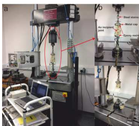
Figure 3. a General view of apparatus set up, b specimen containing an incipient joint during the process of direct tension, c failure pattern of this specimen after direct tension test.
